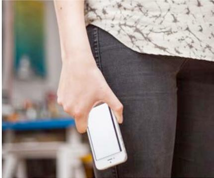
**Figure 1.** The tapper uses accelerometer and gyroscope data from each connected mobile device. Users tap the phone to the drumbeat of the audio performance. This gesture flashes the screen bright white on every detected tap, and sends the tapping rhythm to our main controller. The main controller renders each tap as a white band, revealing a video. Each new user connection subdivides the projected image playing behind the musicians.
